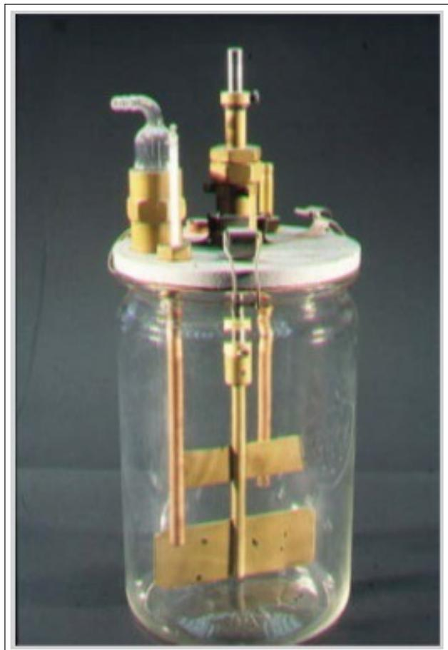
**Figure 8.** The glass reactor in which the first sample of polyethylene was synthesized. (The reactor is on display at the Max-Planck-Institut für Kohlenforschung at Mülheim, Source: [12(a)], Courtesy attributed to: G Fink).
